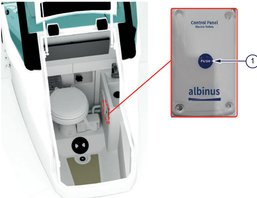
Figure 4.8 - Toilet compartment control panel
